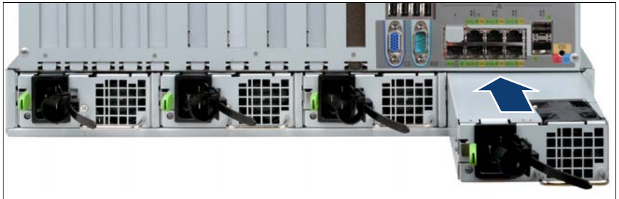
Figure 12: Installing a power supply unit
